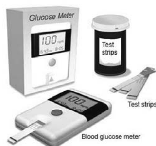
FIGURE 8.5.19 Electronic reading device for glucose strip. The strip is inserted into the side of the machine after the sample has been timed for the reaction to take place and the blood has been wiped off the strip.
