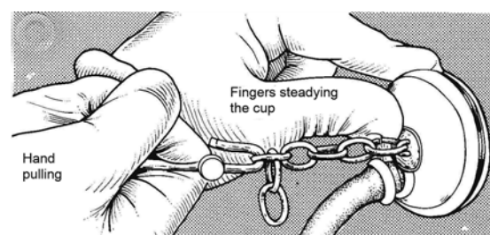
FIGURE 2.13.12 Guiding the cup with the fingers to detect any slippage while pulling.
